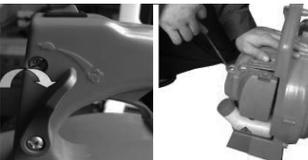
Once warm, the engine should start on the first pull. If it fails to start, re-prime the bulb and ensure the choke lever is in the correct position (Fig.13).
