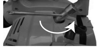
If the spark plug is fouled or is soaked with fuel, clean or replace the plug as required.
