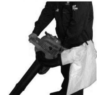
Pull the starter to start the vacuum. Set the throttle setting device at desired speed.
