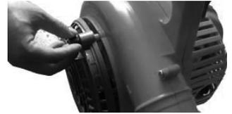
Install vacuum tubes in sequence shown, aligning the grooves on the nozzles with the pegs. Slide the nozzles clockwise onto the pegs(Fig. 5).
