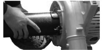
Rotate the connector pipe clockwise to lock, the arrowhead on the connector pipe should be on the same line with the volute case. (Fig. 6).
