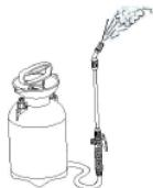
Trial spraying with clean water, and a check of tank, hose, shut-off and nozzle for possible leakage are required prior to operation.
