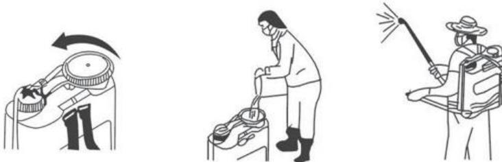
Unscrew the lid of tank and fill it with prepared mixture through a strainer carefully. Then close the tank lid. Mount the sprayer on your back and swing the rocker lever to boost the pressure in the air chamber, and then press the button to spray in spot spraying or continuous spraying form.
