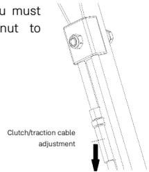
If the brake lever is loose, you must turn the cable adjustment nut to tighten.
