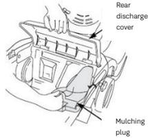
The mulching plug helps to bend the inside of the lawn mower's base for more efficient mulching. Place and remove the mulching plug by lifting the rear discharge guard. The mulching plug only fits one way. Remove it when using the grass bag.
