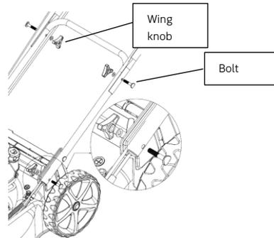
The handle has two height adjustment positions: "L" or "H".
