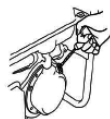
Align the notch on the starter pulley with the hole at the top of recoil starter.
