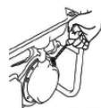
Align the notch on the starter pulley with the hole at the top of each starter.
