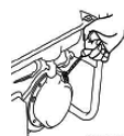
Align the notch on the starter pulley with the hole at the top of the cylinder.
