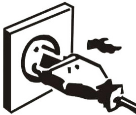
Figure 5: Once the battery is connected to the charger you can connect the charger to a 220V/50Hz socket-outlet.
