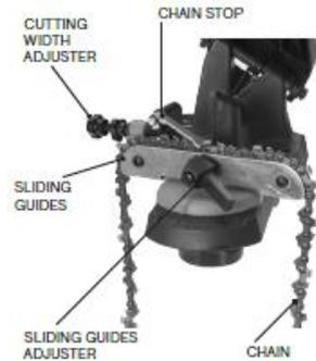
Adjust the spacing of the sliding guides in order to have the minimum clearance for the chain to slide effortlessly.
